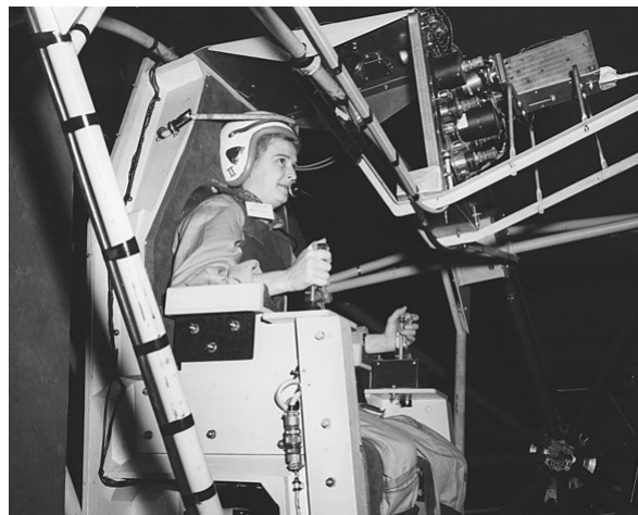
Jerrie Cobb operating the Multi-Axis Space Test Inertia Facility (MASTIF) at the Lewis Research Center in Ohio. This test simulated bringing a spinning spacecraft under control and was one of many that the women of the Mercury 13 went through in order to qualify for space flight. [11]
